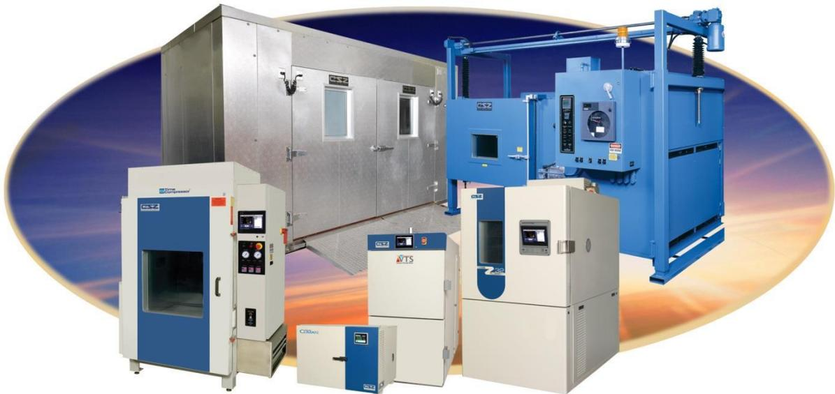
HALT & HASS technology uses a combination of accelerated stresses to expose product flaws early in the design and manufacturing stages, which improves product reliability and customer confidence. HALT & HASS is used to uncover many of the weak links inherent to the design and fabrication process of a new product as well as during the production phase to find manufacturing defects that could cause product failures in the field.
